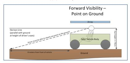
Forward Visibility – (2) A minimum of 10 degrees above the horizon on level ground.
