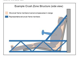
5.2.3 Roll Bar – The roll bar is the structural frame member that extends above the driver's head, protecting the driver in the event of a roll-over. The roll bar must consist of one continuous piece of metal. The bottom of the roll bar must extend at least 5 cm vertically from the top of the driver's head or helmet.
